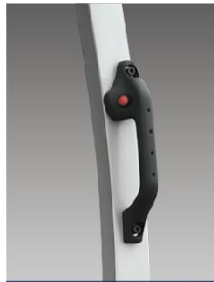
Rear handle with horn ensures stable driving posture when reversing and driving safety and comfort.
